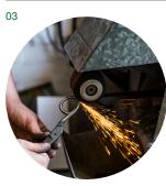
Polishing and filing Every single surface - the blades bows (handles) and shanks (which run between the bows and blades) - is worked upon to smooth and remove "fash" (scale and rough edges).
